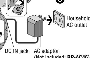
• The battery indicator (
